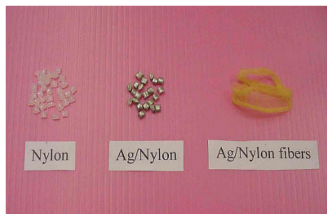
Figure 1 Photograph of nylon chips before and after sonochemical coating with silver and silver–nylon fibers spun from the silver–nylon composite. [Color figure can be viewed in the online issue, which is available at www.interscience.wiley.com .]
